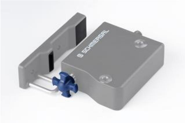
The AZM 300 can be wired in series in conjunction with other Schmersal interlocks through the use of M12 connectors while maintaining SIL 3 / Performance Level E. In addition, the use of a gateway can allow individual annunciation as well as exporting safety data to the plant or machine communication protocol. This allows the designer a number of advantages beyond the obvious ease of wiring such as:
