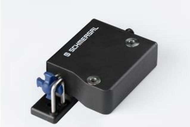
The interlock uses RFID technology in the actuator and as such can utilize a generic actuator or can be “taught” to accept only one actuator. There is also a manual release as well as LED diagnostics located on the body of the interlock. The LED blinking pattern allows an operator to troubleshoot a number of issues such as misalignment, low voltage, high ambient temperature, cross wire- short, etc.
