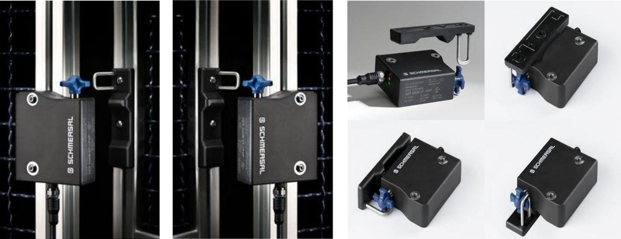
The AZM 300 provides 1000 N of holding force when actuated and can be ordered as power to lock or power to unlock. By a simply turning the blue star handle to either I or II, the designer can achieve 25N or 50N of latching force, eliminating the need for door stops or magnets.
