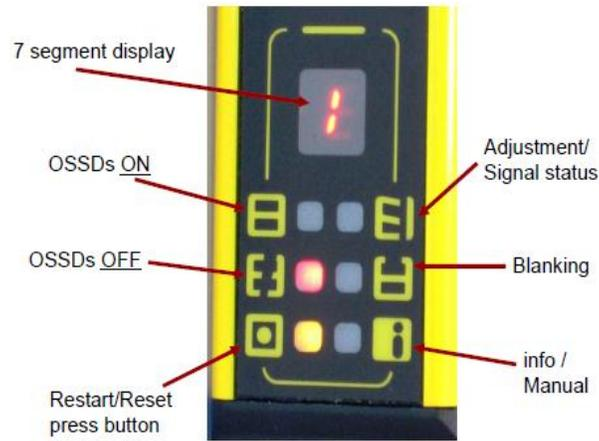
The features and programming could not be more simple. Simply depress the removable push button until the correct parameter is displayed, hold it down for 2.5 seconds, press the button until active or inactive is displayed, hold the button down for 2.5 sec. After your changes have been made scroll to the save function by pressing the button until “S” appears on the display and hold the button for 2.5 seconds.
